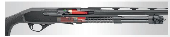
Near the end of the recoil cycle, chamber pressure drops to a safe level and the gun's rearward motion slows. The heavy inertia spring then thrusts the bolt assembly rearward, unlocking the rotating bolt head, extracting the spent shell from the chamber, and pulling it against the ejector.
